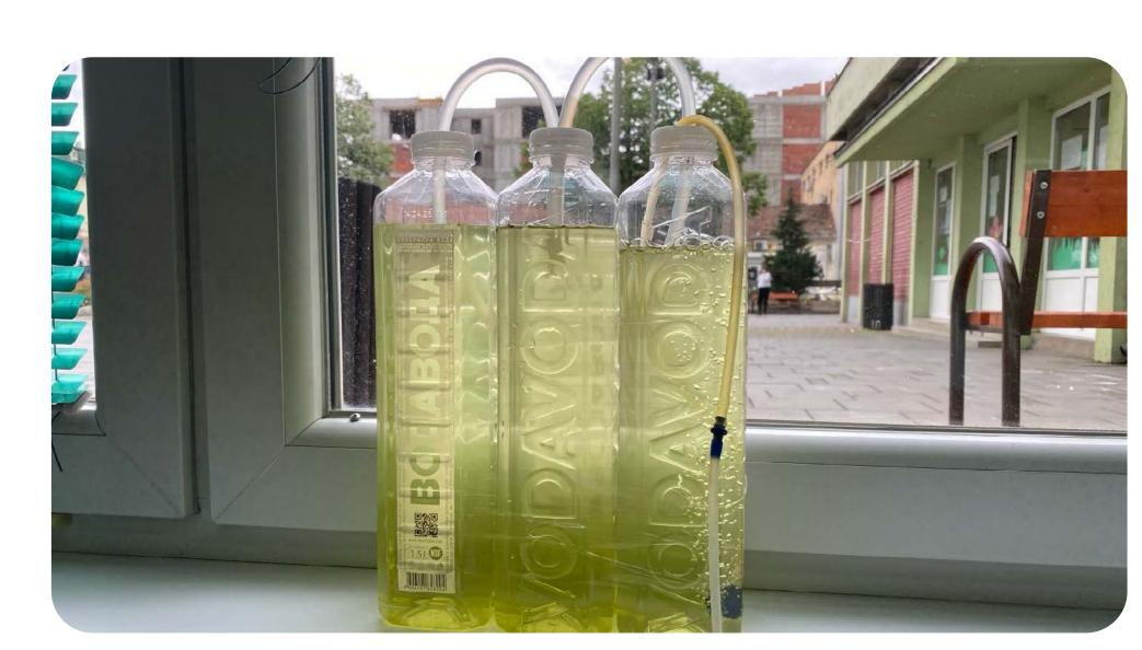
2. A system of connected containers in which air is pumped into the first bottle, then diffuses throughout the entire volume, and finally the oxygen produced during photosynthesis is released through an opening in the cap of the last bottle.
