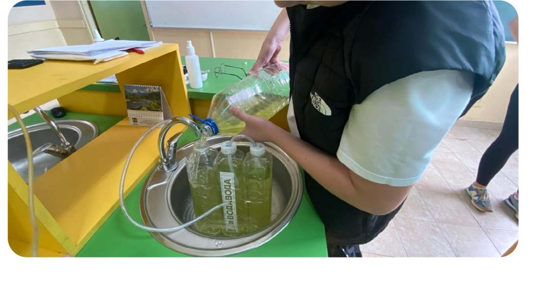
3. A new quantity of algae is added to the reactor every week. In this way, we ensure that the bioreactor efficiently binds CO<sub>2</sub> and aerosol particles, both of which are present in higher concentrations in urban air.
