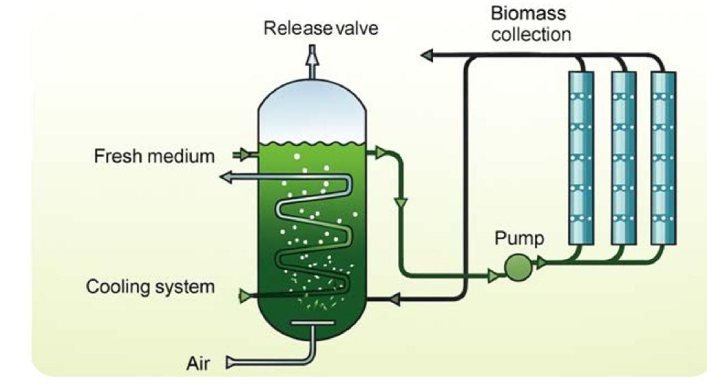
5. Future endevour - a schematic representation of the system for producing and collecting algal biomass in the bioreactor. The image shows that successful algal cultivation requires several components through which the algae pass to be easily collected.
